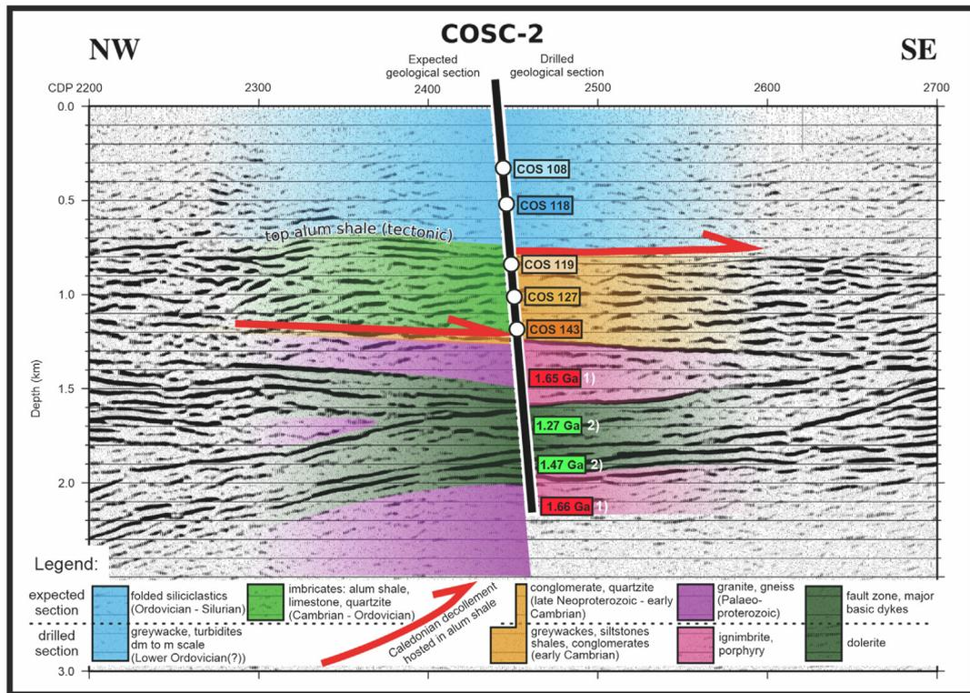
**Fig. 2.** The COSC-2 anticipated geology (left) and the drilled geology (right) superimposed on the depth-converted seismic section that represents the rocks surrounding the COSC-2 drill site (Lehnert et al., 2024; modified from Lorenz et al., 2022 and Hedin et al., 2012). The age data is from Andersson et al. (2022) and Lescoutre et al. (2022).
